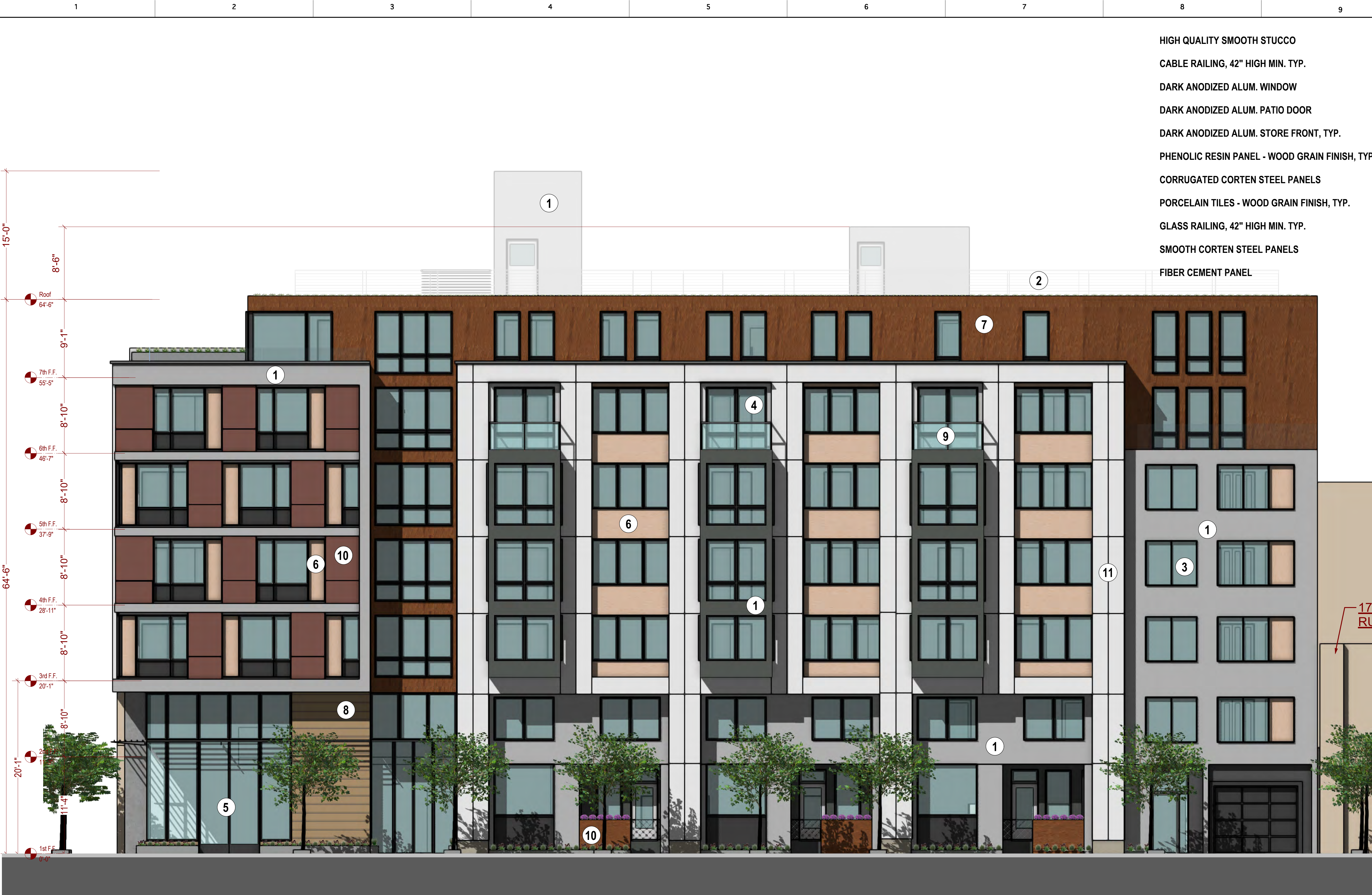
Proposed Right Elevation (Russ Street) 3/16" = 1'-0"
