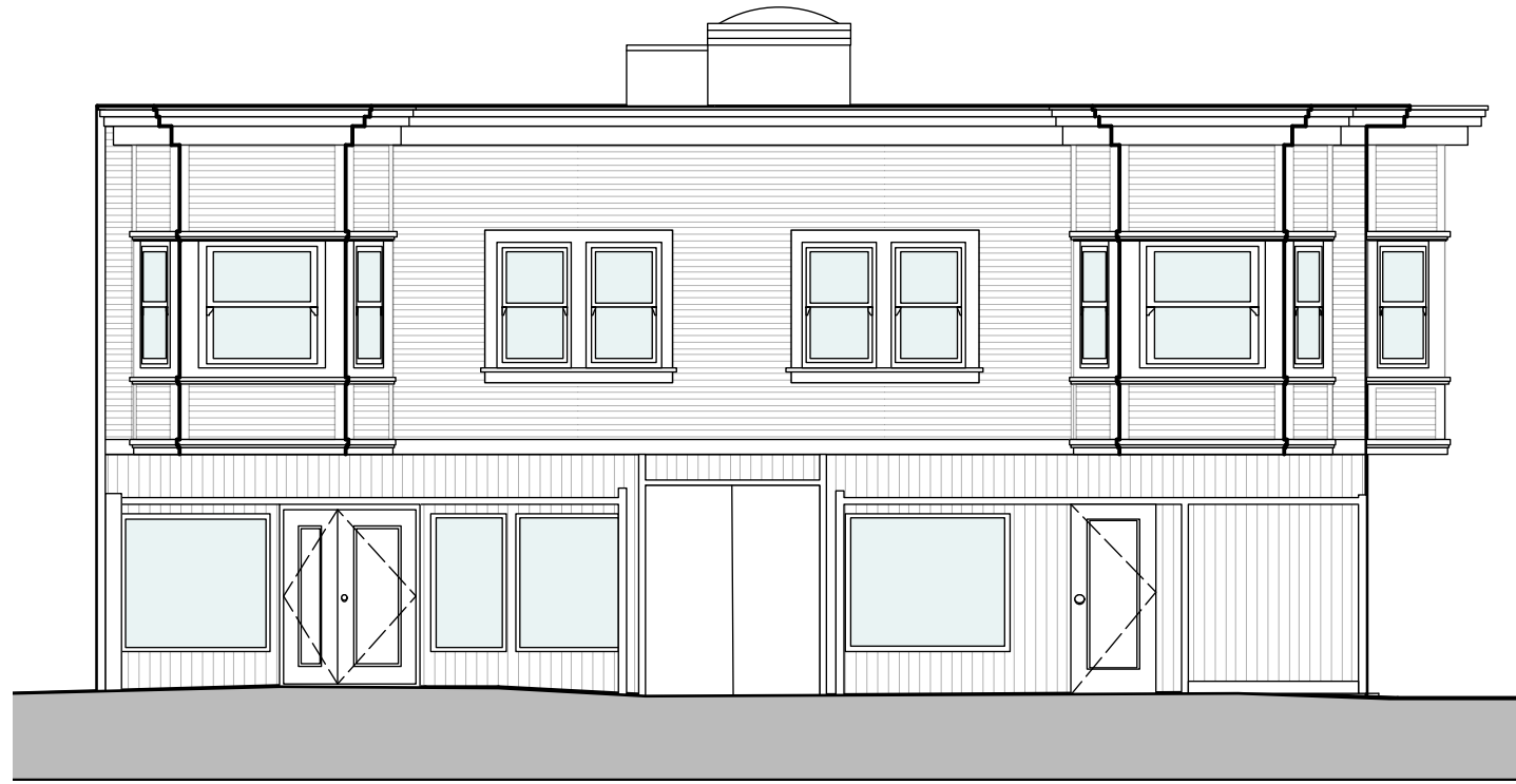
Existing Front Elevation (Folsom St) 1/8" = 1'-0"
