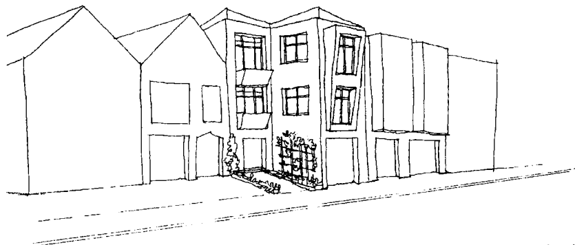
The subject building uses an alternative method of averaging the front setback (Planning Code Section 132(b)) to unify the streetscape.
