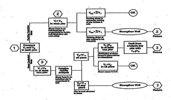
V<sub>r</sub> = Rocking shear capacity of pier.
