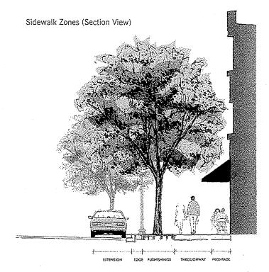
As the furnishing zone acts as a buffer between pedestrians and the roadway, the width of the furnishing zone should be based upon traffic speeds and volumes and whether on-street parking is provided. If no on-street parking is provided and traffic speeds are 25 mph or less, the furnishing zone dimension should be a minimum of 4 feet in width. For speeds of 30 mph or above, the furnishing zone should be one foot wider for every 5 mph increment in posted speed above 30 mph.
