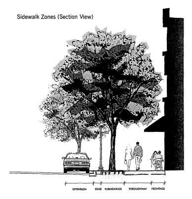
As the furnishing zone acts as a buffer between pedestrians and the roadway, the width of the furnishing zone should be based upon traffic speeds and volumes and whether on-street parking is provided. If no on-street parking is provided and traffic speeds are 25 mph or less, the furnishing zone dimension should be a minimum of 4 feet in width. For speeds of 30 mph or above, the furnishing zone should be one foot wider for every 5 mph increment in posted speed above 30 mph.
