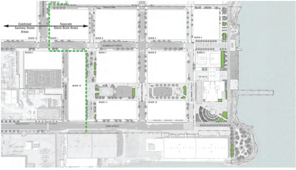
Figure 4.7.1 Stormwater Management and Conceptual Layout of Bioretention Treatment Areas
