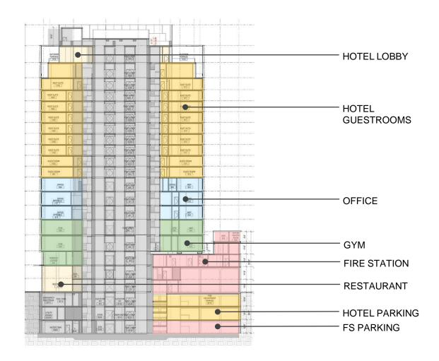
Section Diagram, Fire Station footprint in red
