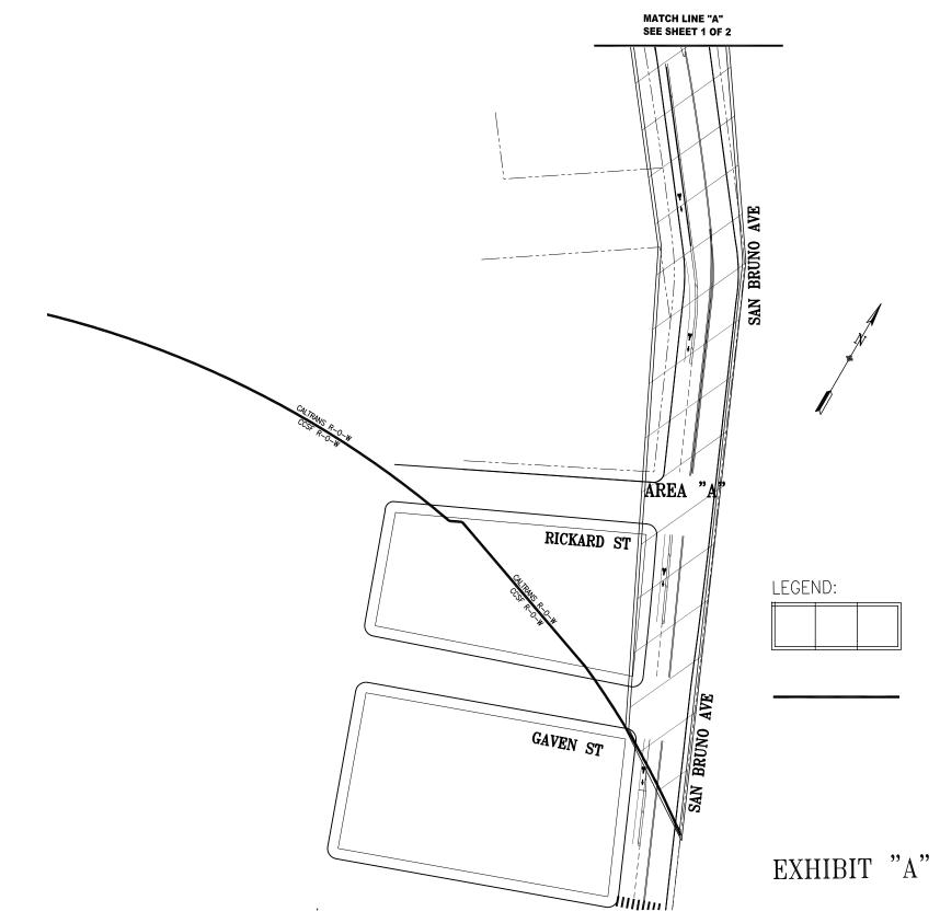
CCSF SHALL MAINTAIN ALL PAVEMENT MARKINGS AND STRIPING INCLUDING BICYCLE PATH AND LANE AND CYCLETRACK MARKINGS AND FLEXIBLE DELINEATORS IN AREA "A"
