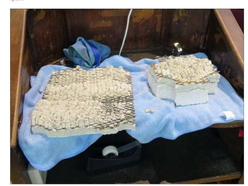
${\it Plaster from Probe 1 and Probe 6. Note the presence of a distinct scratch coat and brown coat.}$
