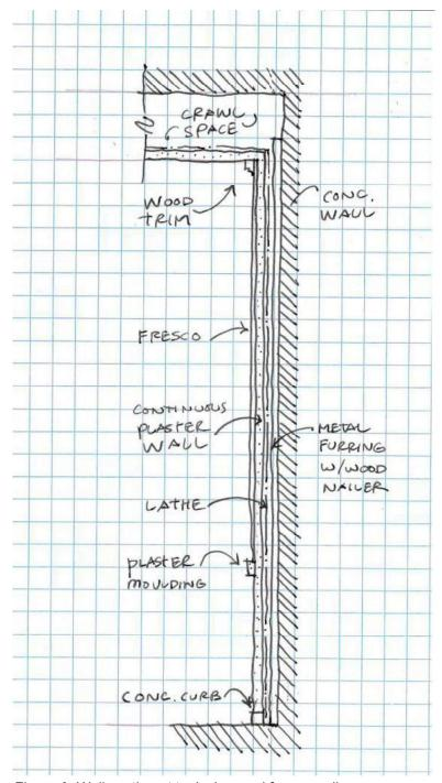
Figure 6: Wall section at typical curved fresco wall
