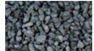
3/4" minimum crushed black basalt
