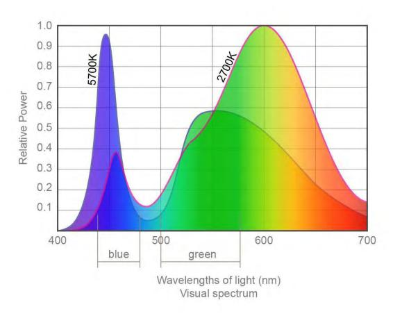
Notice that the peak of the 5700K source is close to the peak sensitivity of the circadian system shown in Figure 1 in section 1.1.1
