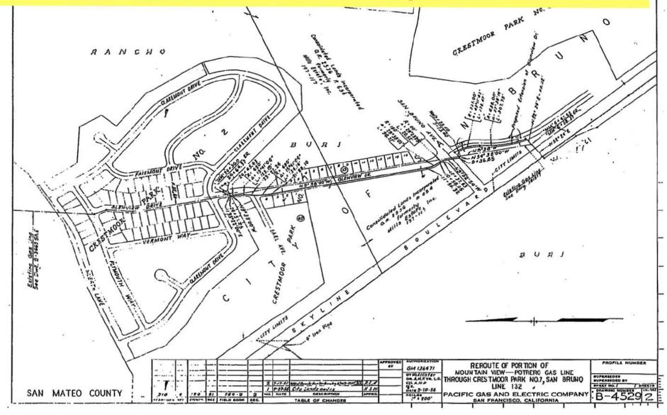
PG&E did not provide the construction 'details' to accommodate the change in vertical direction at the bottom of the 'ravine'
