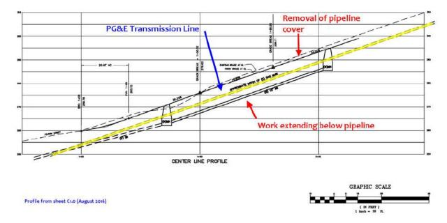
Figure 6: Plans call for removal of pipeline cover as well as construction work <u>below</u> the existing pipeline.
