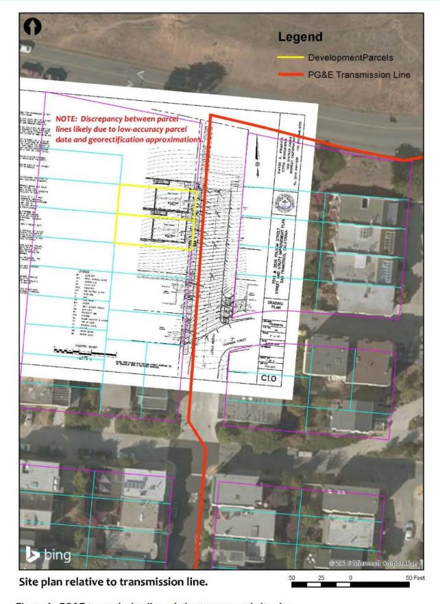
Figure 4: PG&E transmission line relative to proposed site plan.
