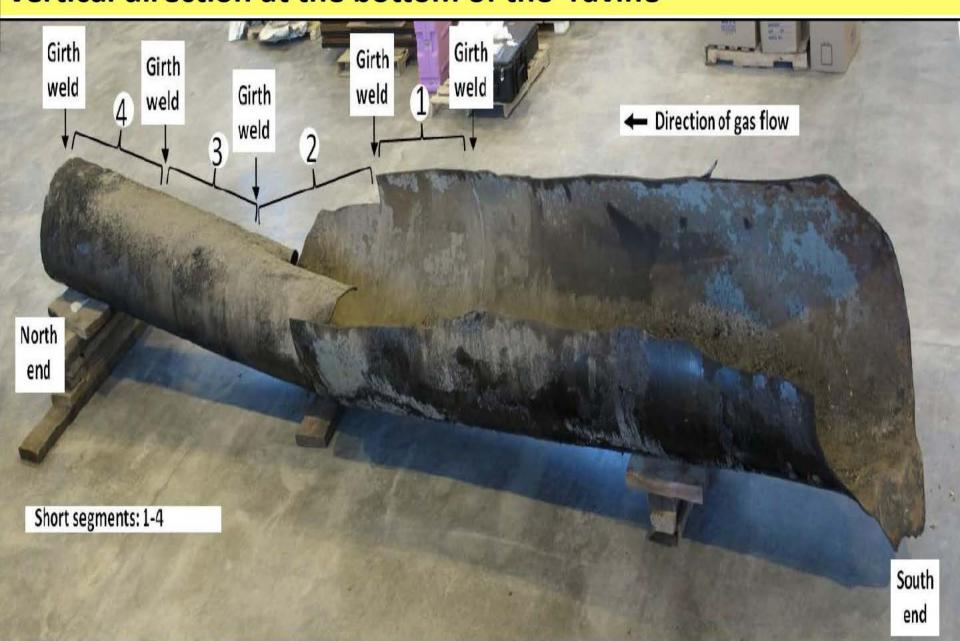
Longitudinal welds inside pipe missing
