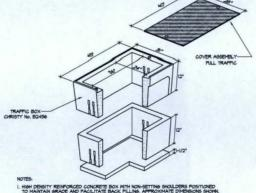
High DENSITY REINFORCED CONCRETE BOX WITH NON-SETTING SHOULDERS POSITIONED TO MAINTAIN GRADE AND FACILITATE BACK FILLING, APPROXIMATE DIMENSIONS SHOWN
