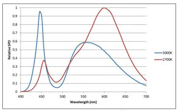
Notice the larger peak in the 440-450 nm range with the 5000k (cooler) LED source, as opposed to the 2700K (warmer) LED source. This is significant for scotopic sensitivity as well as melanopic sensitivity.
