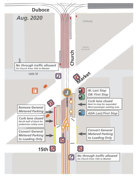
Figure 4: Proposed Phase 1 J Church Terminal and Transfer modification
