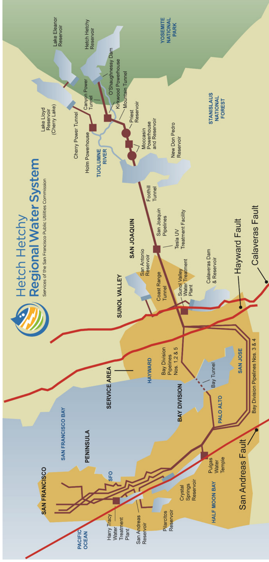
Figure 1-1 (Not to Scale) – The above map depicts the Hetch Hetchy Regional Water System, which delivers water approximately 160 miles from the Hetch Hetchy Reservoir to San Francisco. The Water Enterprise consists of over 1,235 miles of pipeline, 11 reservoirs, six groundwater wells, eight storage tanks, 24 pump stations, eight hydropneumatic stations and 17 chlorination stations located within the San Francisco city limit and further comprises over 389 miles of pipeline, over 74 miles of tunnels, 11 reservoirs, 13 groundwater wells, five pump stations, and three water treatment plants located outside of San Francisco. For further description of the SFPUC's Water System, see "THE WATER ENTERPRISE."
