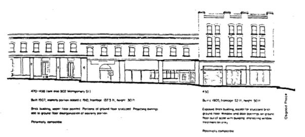
Figure 4: Façade elevations and architectural description diagram for the block of the subject building (subject building at right). Source: Jackson Square Report.
