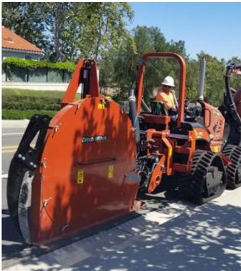
Faster, lower impact method. 16"-24" depth trench cut, 8-9" offset from concrete gutter.
