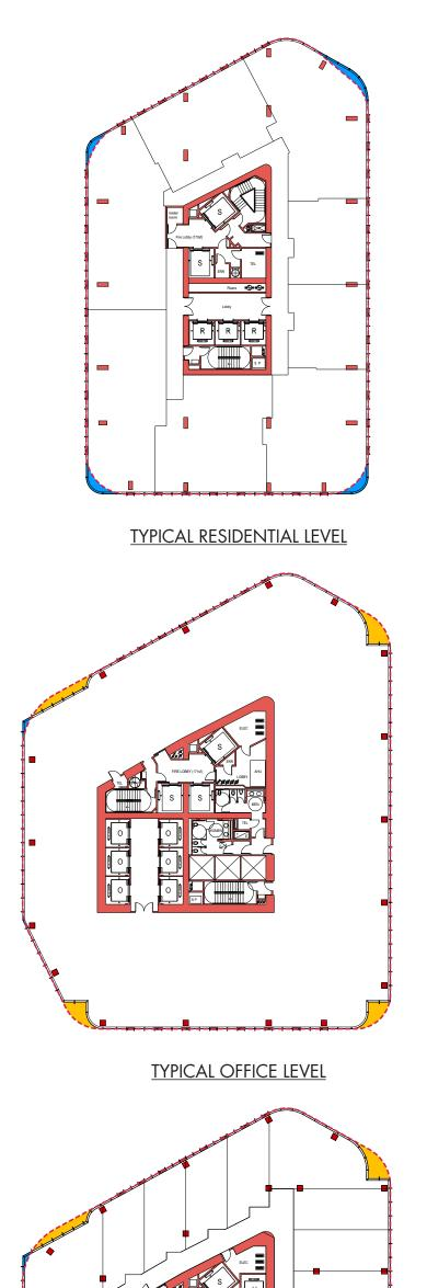
PREVIOUS FLOOR PLATE: 15,000 SF REVISED FLOOR PLATE: 15,305 SF 305 SF ADDITION PER FLOOR PLATE
