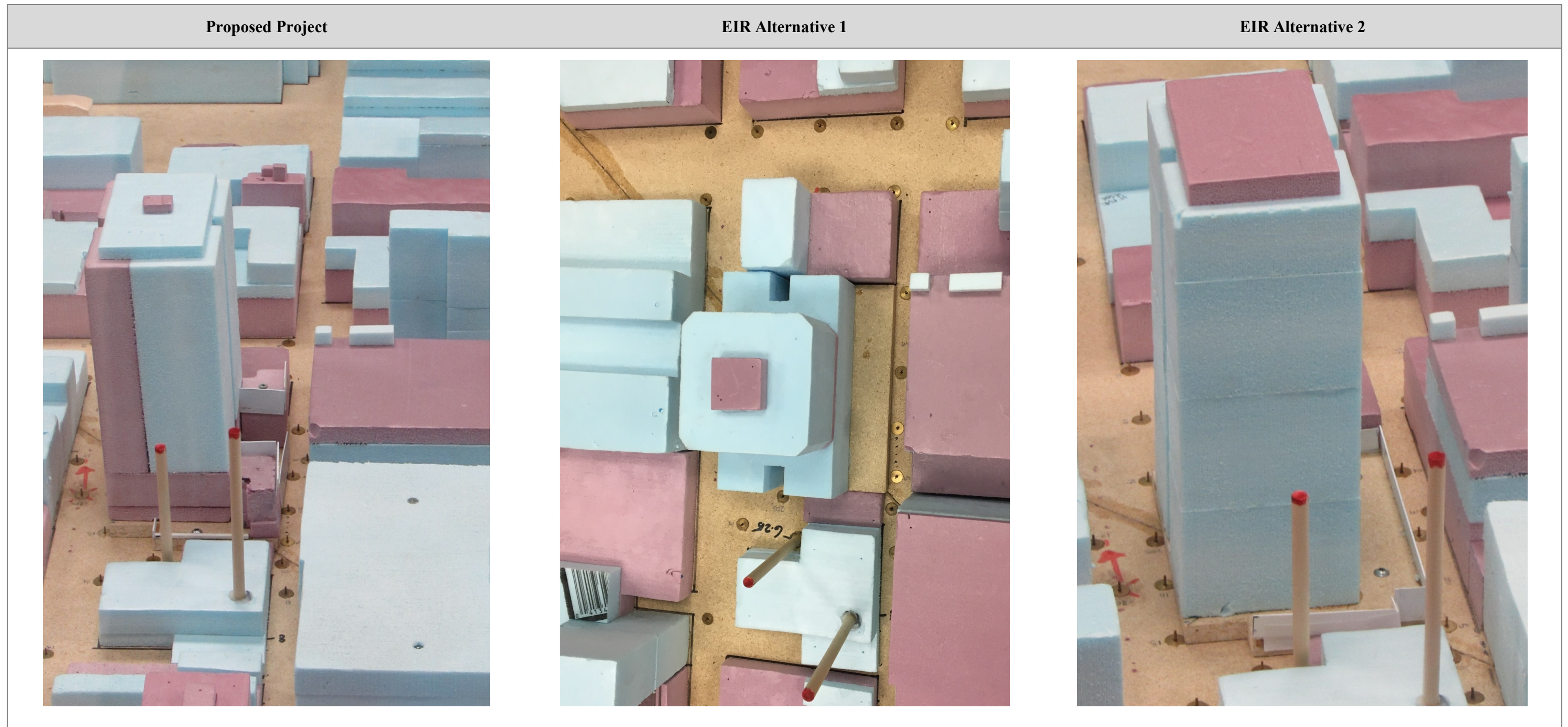
Figure 15: Wind tunnel model of the Proposed Project (left), EIR Alternative 1 (center) and EIR Alternative 2 (right)
