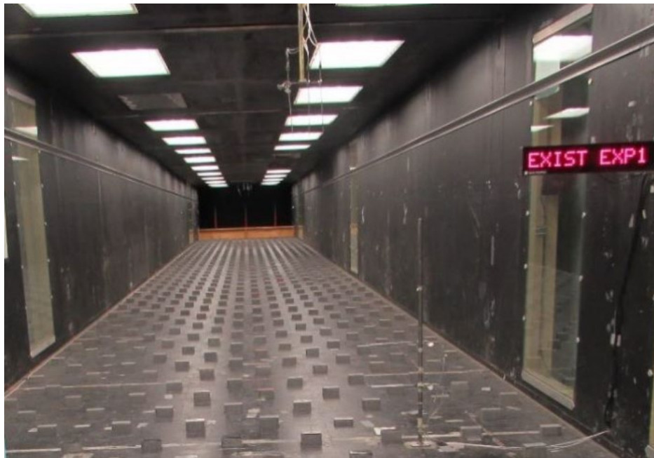
Figure 9: View of the wind tunnel model upwind of the site model
