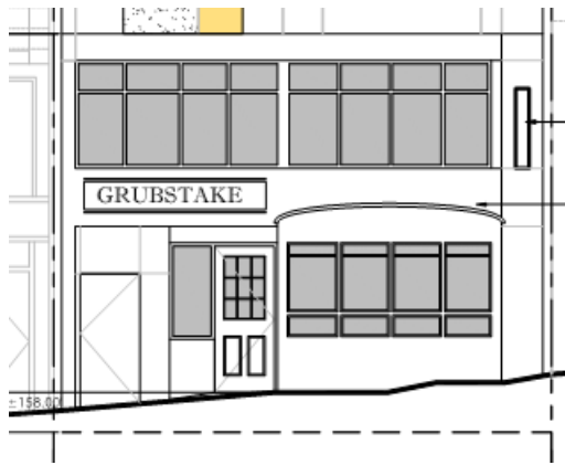
Revised: Existing windows including green toplites are being salvaged for reinstallation in the lunch wagon façade.
