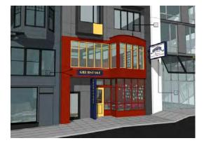
Original: The original design had the arched lunch wagon façade located on the second floor. The façade was at an angle to the property line and did not match the existing footprint.
