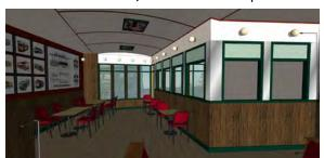
Original: The barrel vault ceiling is not symmetrically defined. The globe lights are inconsistently placed and located on walls outside the barrel vault. The lunch wagon is not defined by unique finishes or colors.
